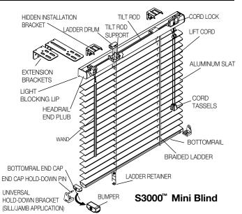
Slat thickness and ladder support distances shall be such that there is no visible sag.
