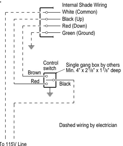
NOTE: This wiring diagram is for standard right-hand motor placement, fabric from rear of roller. It also applies for left-hand motor placement, fabric from the front of the roller. For left hand motor placement with fabric from rear of roller, or right hand motor placement with fabric from front of roller, Red becomes "Up" and Black becomes "Down."
