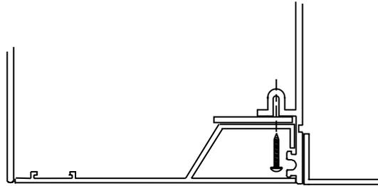
Dual Roller Headbox End Bracket—Side View
