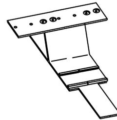
Bottom Closure Center Bracket for Multiple Rollers in Front or Back
